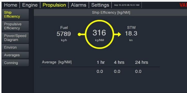
Figure 37 – Propulsion Ship Efficiency screen
